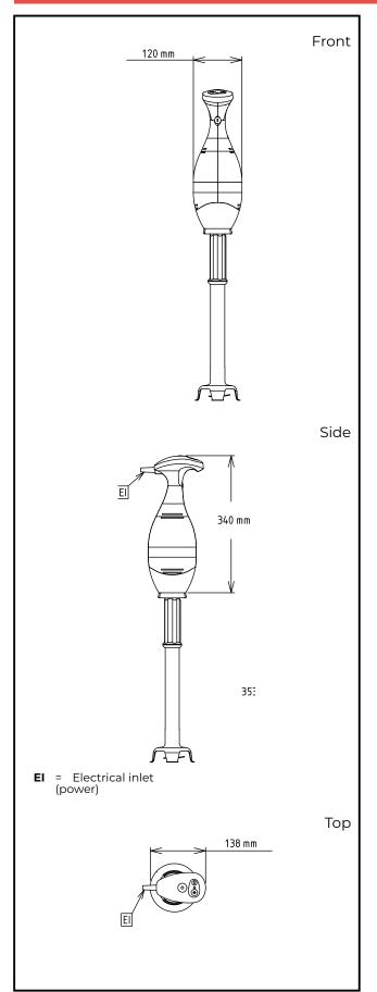
Electric Supply voltage: 220-240 V/1 ph/50/60 Hz **Electrical power max:** 0.65 kW 0.65 kW **Total Watts:** Key Information: External dimensions, Width: 138 mm External dimensions, 120 mm Depth: External dimensions, 340 mm Height: **Shipping weight:** 3.7 kg
